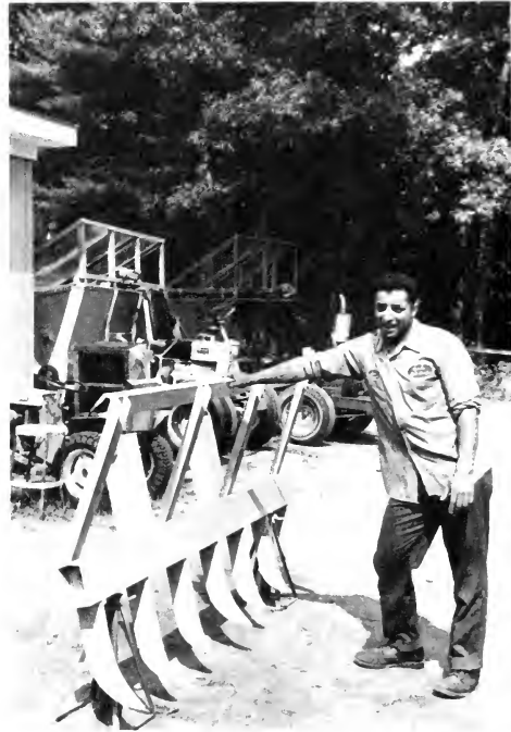
A heavy duty rake which can be attached to standard equipment to speedily dig up old bogs and prepare them for replanting.
